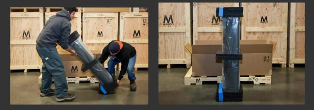
Using two people, one to steady the top of the speaker on the floor and one to lift the bottom of the speaker; stand the speaker, in its foam, onto its top.
