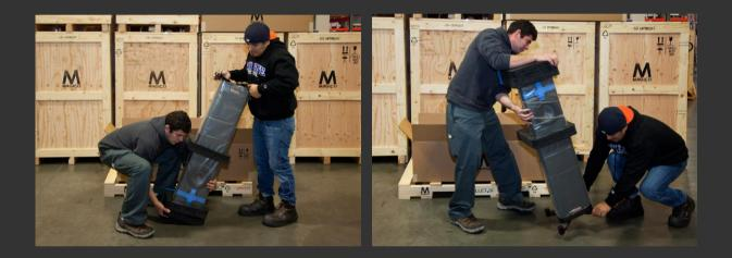
With one person lifting either end of the speaker carefully flip it on to its feet. If you have hardwood or delicate floors, lay down a protective mat.
