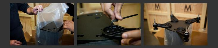
Remove the protective plastic from the bottom of the speaker. Using the provided 3/16" hex Allen key tighten each foot to the bottom of the speaker using three bolts each.
